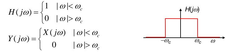
The filter's impulse response is the inverse Fourier transform
